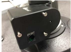
7. Connect the eFocuser to the mount use supplied 6P6C cable (same as the hand controller cable.) One end to the iPORT on the eFocuser. The other end to the PORT on an iOptron mount.
