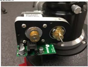
3. Put the eFocuser pulley onto the dual-speed focuser tuning shaft. Tighten the set screw to secure it onto the fine tuning shaft.
