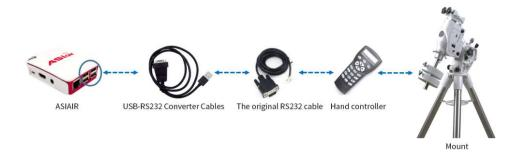
CEM25P/EC, ZEQ25, iEQ30, iEQ45, etc. When using serial port connection, two data cables are required to connect ASIAIR and equatorial mount hand controller (as shown above). Select the corresponding equatorial mount model in ASIAIR's equatorial setup with a baud rate of 9600.
